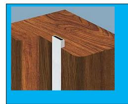
Intumescent strips fitted to the **door** frame – because there are no cold smoke seals it is permissible to paint over the intumescent strips with a maximum of five coats of conventional paint or lacquer or a maximum of 0.5 mm, whichever is the greater.
